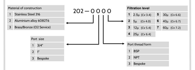
Example part number: 202-3214: Brass/bronze construction, female 1" BSP ports, 25µ filter
