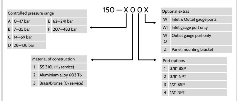
Example part number: 150-F11: 207-483 bar control range, Stainless steel construction, female 3/8" BSP ports, no extras
