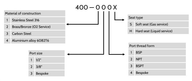
Example part number: 400-110S: Stainless steel 316 construction, female 1/2" BSP ports, soft seat.
